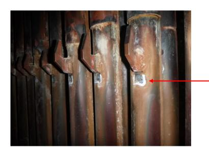
16 (last tube) located underneath the alignment lugs due to IK -19.
