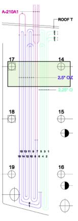
Tube Material: 2.25" O.D. x 0.220" MWT SA-210 A1
